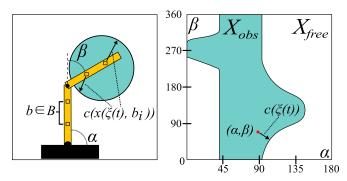
Fig. 2. Both figures show a 2D manipulation problem in a planar space and how the environment of given problem looks different in the workspace (left) and the configuration space (right). In the workspace, a robot arm is simplified by a set of body points  $b \in B$  (small squares); its potentials against the obstacle circle are computed by the proximity of those in the workspace (black arrow). The right figure shows the same circumstance, but in the configuration space.
