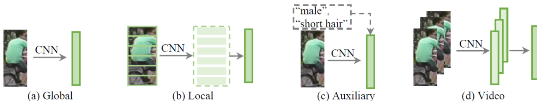
Fig. 2: Four different feature learning strategies. a) Global Feature, learning a global representation for each person image in § 2.1.1; b) Local Feature, learning part-aggregated local features in § 2.1.2; c) Auxiliary Feature, learning the feature representation using auxiliary information, e.g. , attributes [62], [63] in § 2.1.3 and d) Video Feature, learning the video representation using multiple image frames and temporal information [64], [65] in § 2.1.4.
