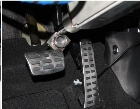
Brake & Throttle Control Actuator
