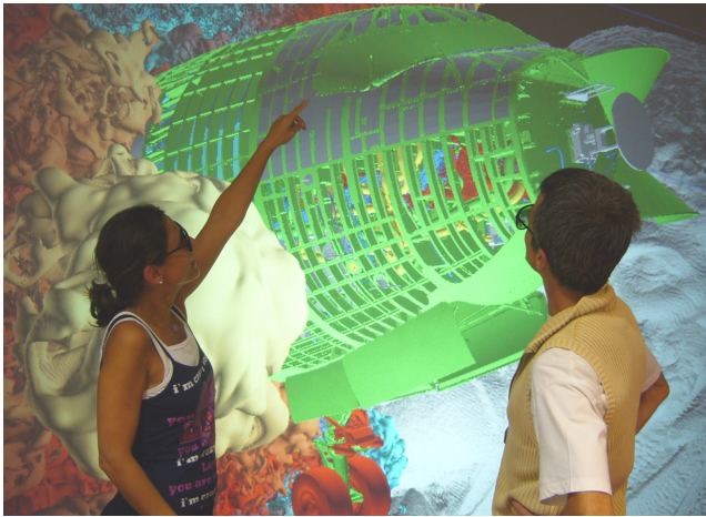
Fig. 14. Far Voxels Rendering Example. A 1.2 billion triangles scene interactively inspected on a large scale stereoscopic display driven by single PC, which renders two 1024 \times 768 images per frame with a 1 pixel tolerance.
